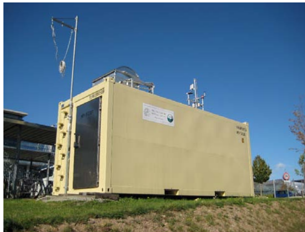
Figure 2.1: Picture of the MPI-BGC FTIR container at its preliminary location close to the MPI-BGC in Jena.
