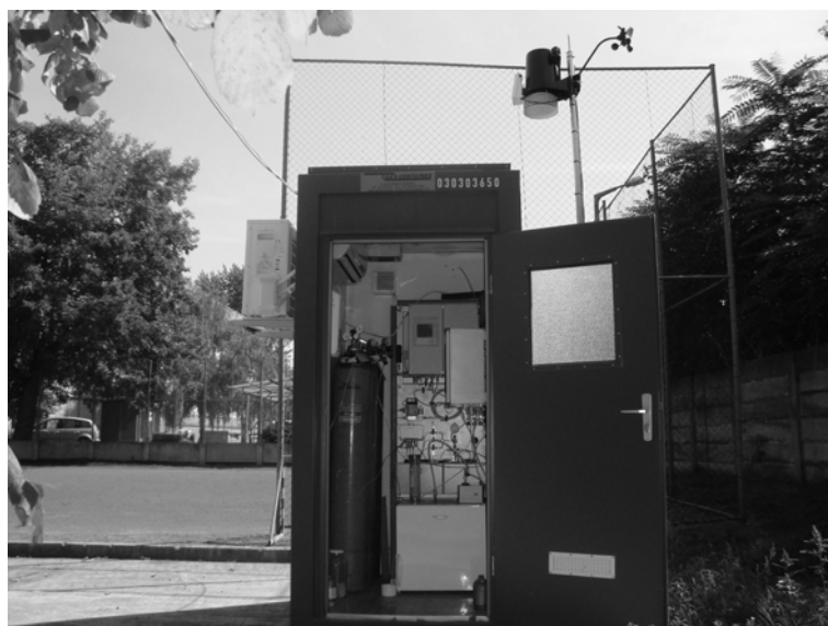
Figure 2. Photo of the developed field deployable fossil fuel CO 2 monitoring station.
