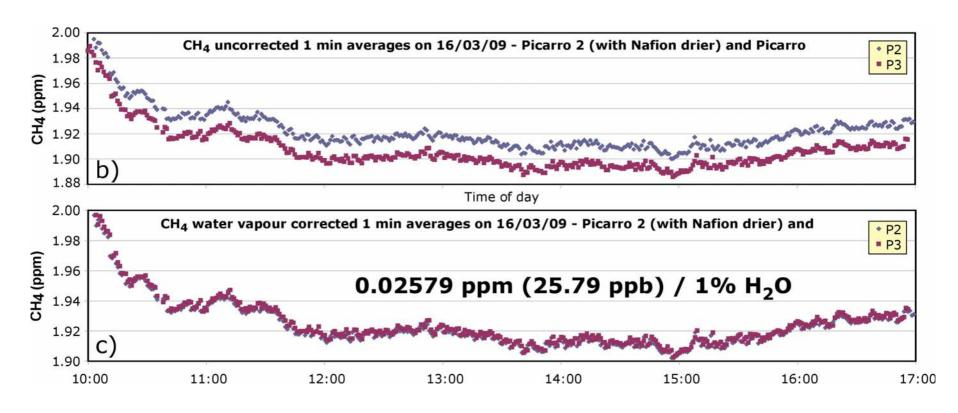
Validity of the correction established for CH4: comparison at Mace Head between the AGAGE GC (data from S.O'Doherty) and the Picarro (non-dried air)
