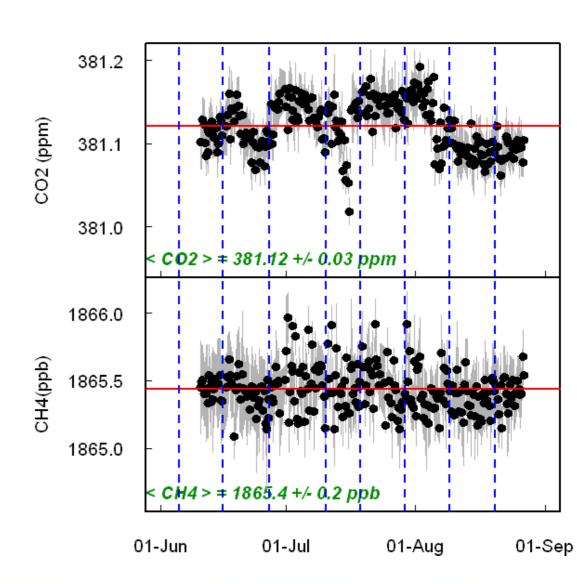
Tests at LSCE in 2008: check validity of Picarro water correction for CO2
