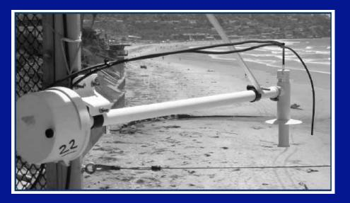
Heating of unshielded inlet drives thermal fractionation of Ar/N<sub>2</sub> Aspirator fan provides 5m/s flow past tubing intake
