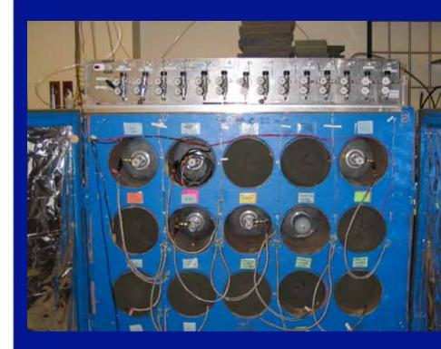
For  $O_2/N_2$ , Ar/N<sub>2</sub>: must dispense standard gases from horizontal position in insulated enclosure
