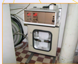
Atmospheric 14 CO 2 sampling unit with two lines (developed by ATOMKI)
